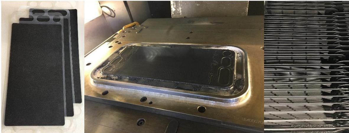
Figure (left-to-right): MEAs in the new design, casting of BPP and flow-plates ready to ship.
