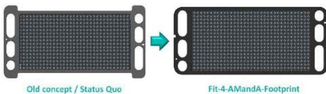
Figure 1: Redesign of the BPP for automated machine handling
