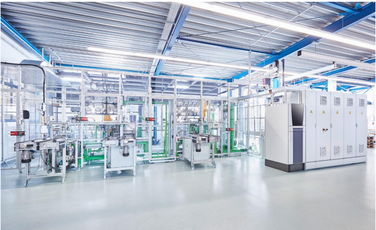
Figure 17: Complete stack assembly system (MMM)
